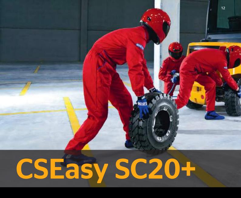
With the unique mounting, you benefit two-fold. For one, it makes you independent from mounting presses and external services. This is made possible by the CSEasy adapter, which can be loosened with a simple Allen key. Compared to conventional solid tires, the adapter ensures a significantly more secure rim seating and simultaneously prevents the tires from twisting on the rim.
