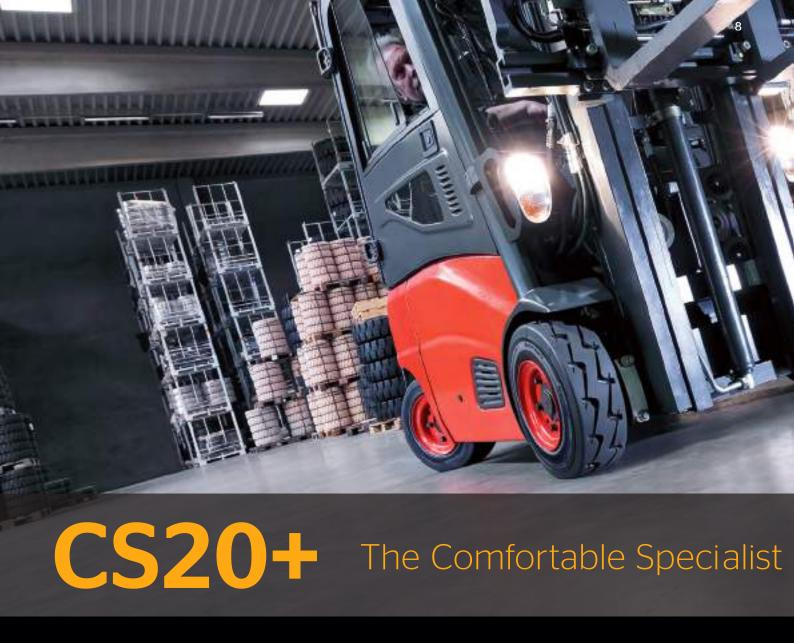
The CS20 has always been an extraordinary solid tire; By means of the new Continental Plus Compound, it becomes even better in the shape of CS20+. Its unique double-L profile with closed shoulders ensures not only an exceptionally precise steering- and cornering behavior, but also minimizes vibrations at the same time for excellent driving comfort.
